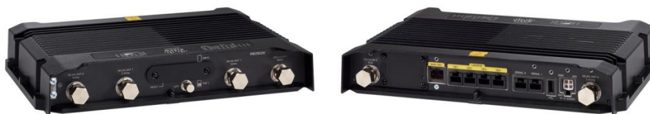
Figure 1. Cisco 829 Industrial Integrated Services Router with 4G LTE and Dual 802.11n a/g/n (WiFi) Radios
